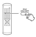
The DVI ON/OFF button turns output from the DVI output on and off. In order to use this output, a DVI/HDCP-compliant television must be used.
